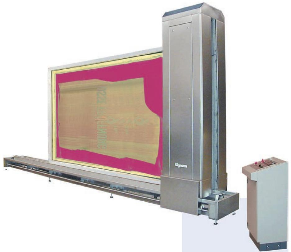
Linear developing tower with nozzle holders on both sides
